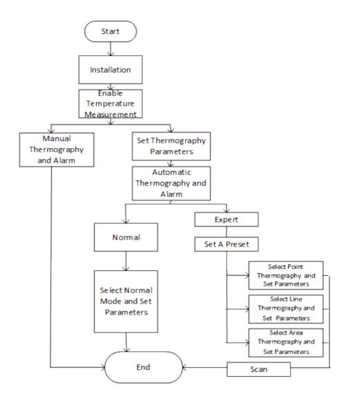
Figure 3-1 Thermography Configuration Flow Chart
