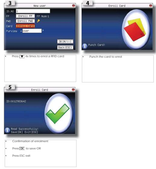
\* RFID card is for added security on the unit, or if the user can't use a fringerprint
