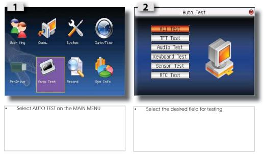
\* Ensure to run a AUTOTEST to test all functions on unit
