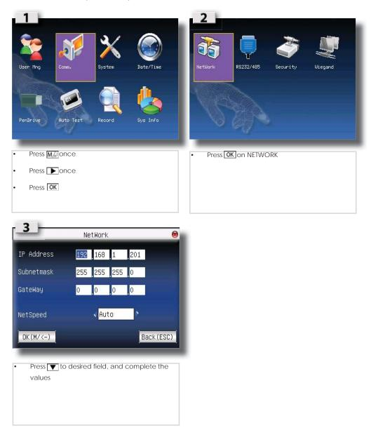
\* Ensure to assign a static address, units will not work on DHCP
