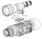
FIGURE 2-9. MOUNTING AN IR ILLUMINATOR
