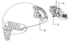
FIGURE 2-4. MOUNTING THE HELMET MOUNT FOR A SHROUD
