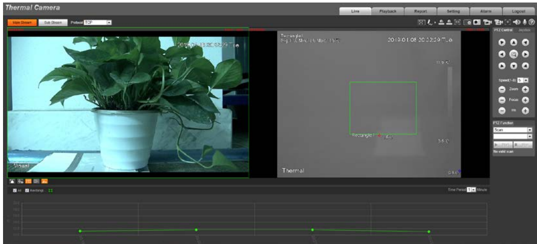
Figure 3-6 Temperature recording area
